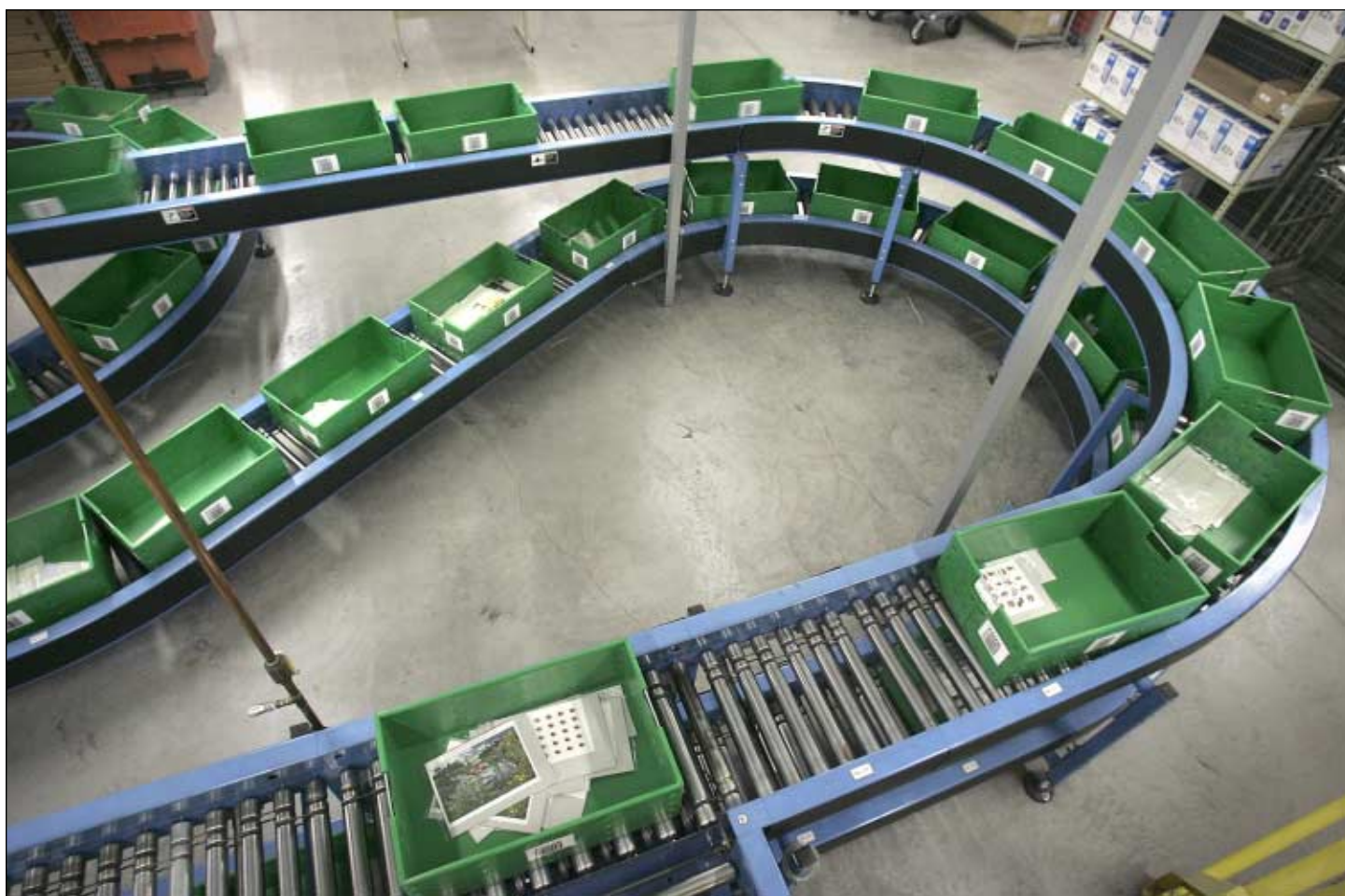
At the U.S. Postal Service's Stamp Fulfillment Services, 12,000 to 15,000 orders per day are filled with computer-controlled conveyor belts.
